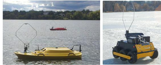
Fig. 1. (Left) Two robotic boats tracking invasive fish in Minnesota lakes. (Right) Rovers used in winter experiments when the lakes freeze over.
