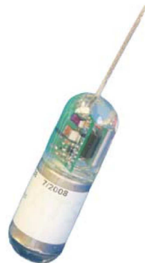
Figure 4: The transmitter used for tagging fish. It is 85mm long and 15mm in diameter. Image from ATS Track.
