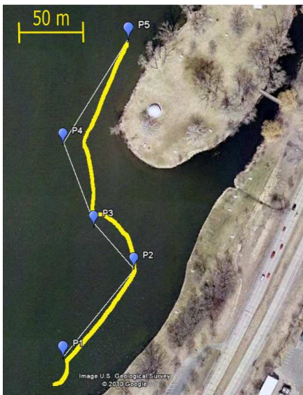
(a) The GPS trail is marked in yellow along with the reference trajectory in white. The total distance covered from the first to the last waypoint was about 304m in 16 mins.
