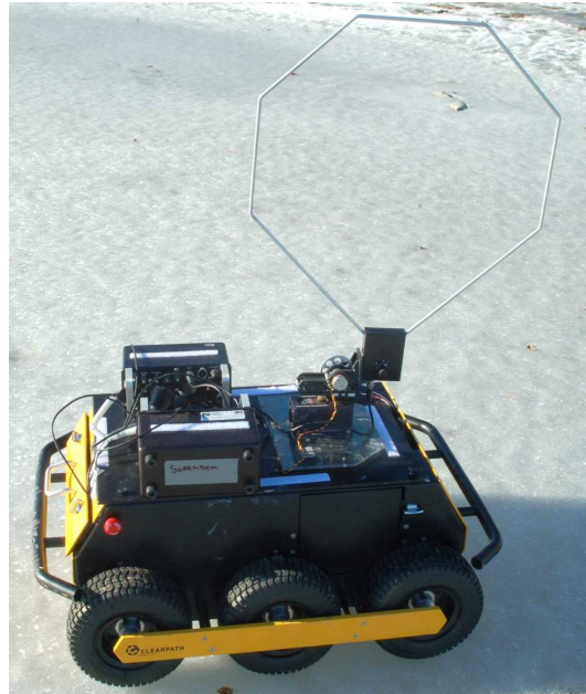
Fig. 1. The mobile robot, loop antenna, and sensing equipment. The picture was taken during field trials on Lake Gervais, MN.
